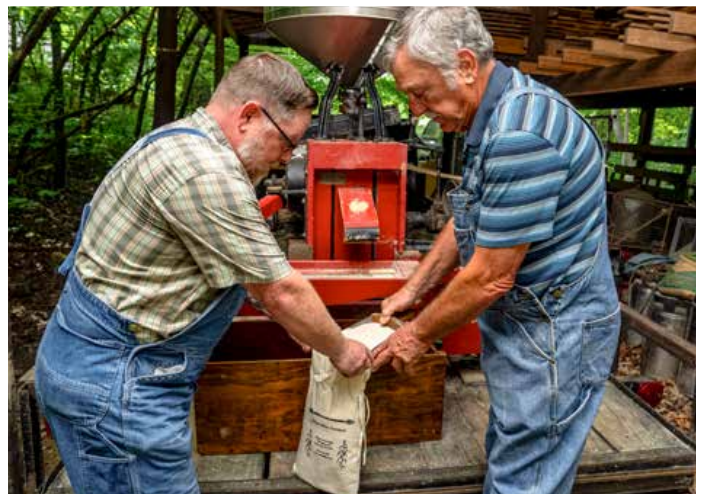
TOP: The gas-powered grill uses special stones to grind the corn.
