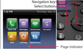
To get to different icons, you can use the right, left, up, and down arrow keys on the Navigation key (shown above right). To choose an icon, press the **Select** button in the center of the Navigation key.
